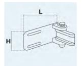
Fitting no.3 Straight fitting in stainless steel. Used on bathing chairs
