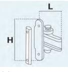
Fitting no.7 With this fitting the side support cannot be adjusted in width, which makes it important to choose the correct bar
