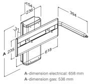
Materials: Aluminium, powder coated stainless steel, synthetic and plastic PS Max. load: Wash basin brackets PLUS and COMFORT: 100 kg. SELECT: 150 kg. Brackets: 150 kg.
