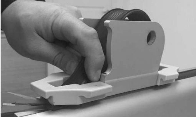
Thread the rubber profile as shown in the photo
