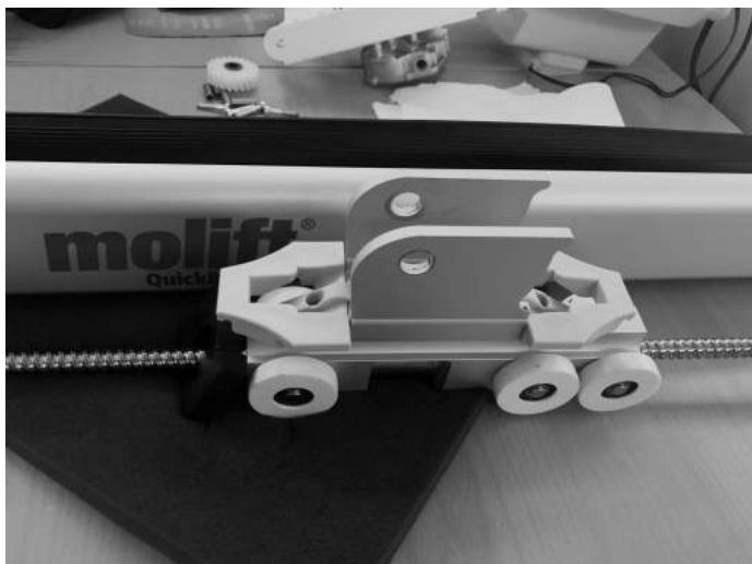
Pull driveline out of profile
