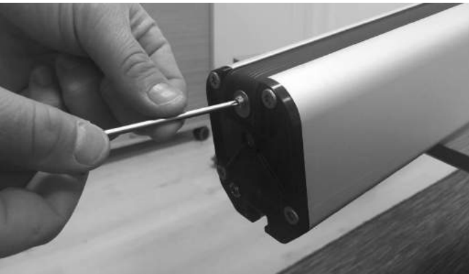
Remove screw and washer (T20)
