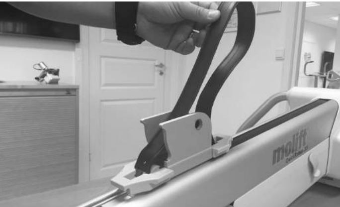
Pull the rubber profile out from trolley and column.
