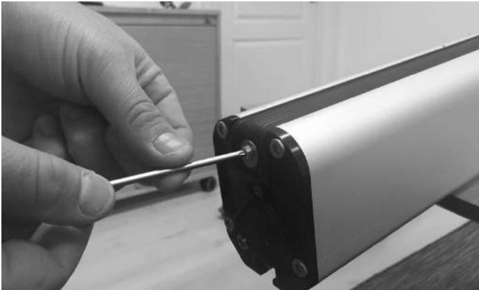
Reassemble screw and washer (T20)
