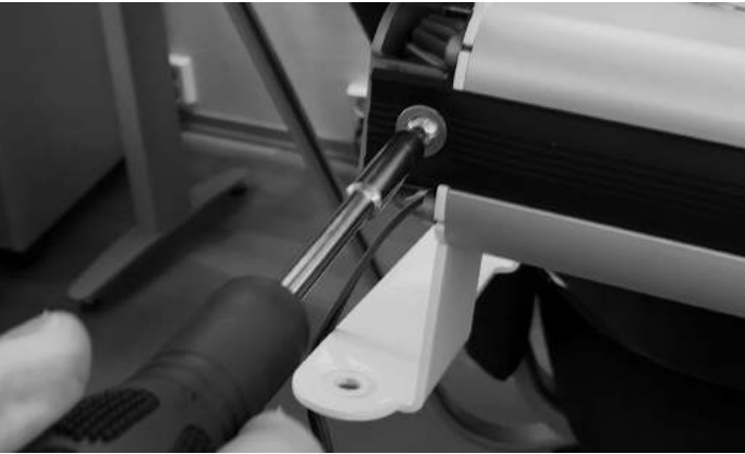
Remove screw from rubber profile (T15).
