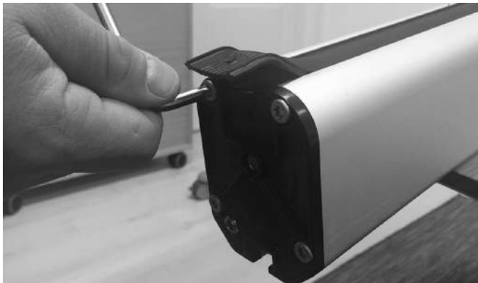
Remove 4x T30 screws from bottom cover
