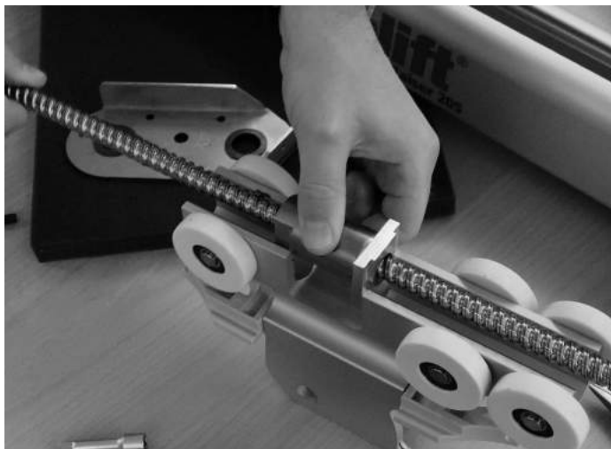
Lift trolley out from ball screw nut to replace trolley og ball screw (driveline)
