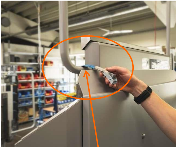
Ensure tension belt is threaded up over the top of the safety bar.
